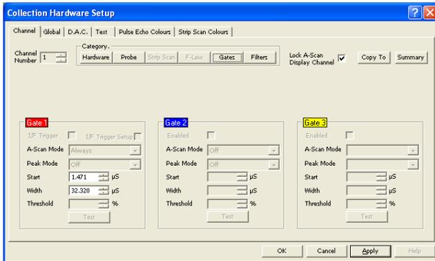
TOFD channels only have 1 data collection gate, and are drawn in RED on the A-Scan display.
