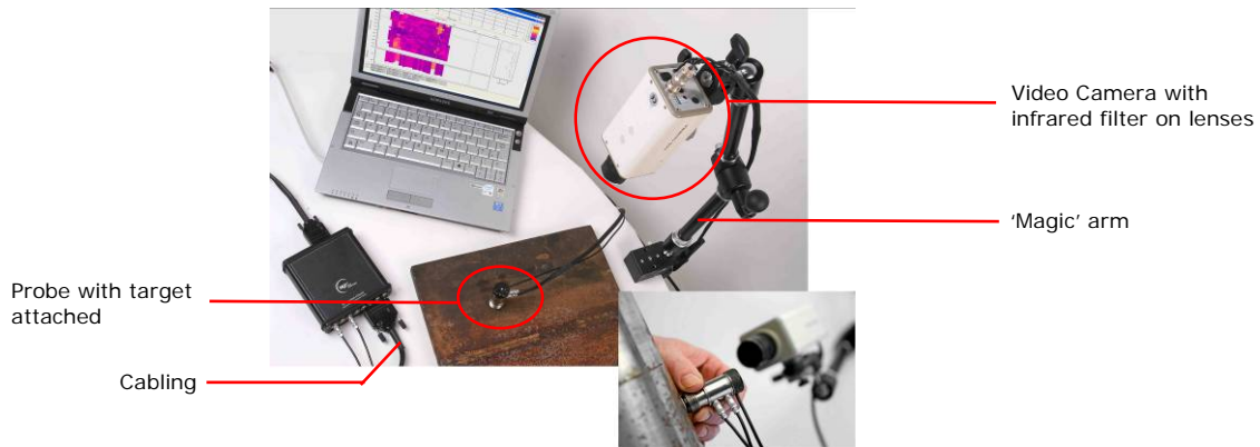
TD Corrosion Mapping Kit connected to a TD Pocket-Scan
