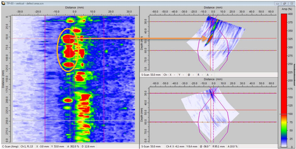
Fig.6 PAUT scan image with weld discontinuity
