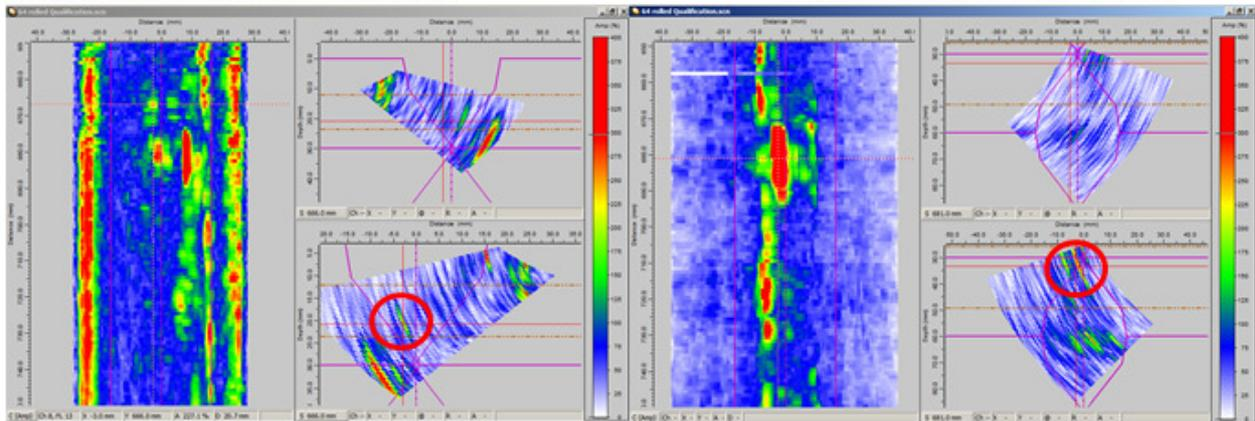
Fig.5 PAUT qualification scan image with embedded artificial reflector
