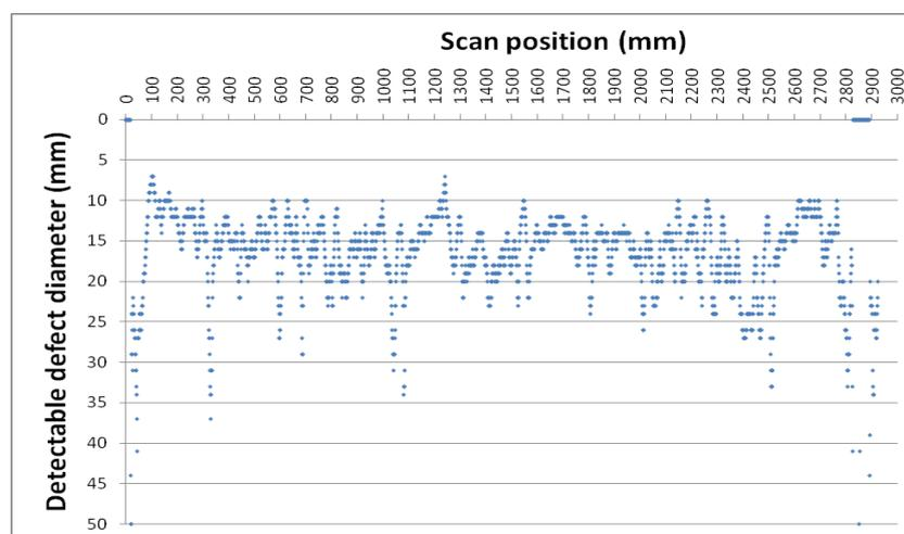
Figure 9. Example of a (field data) sensitivity graph in terms of minimum detectable wall loss area diameter instead of SNR, using a conversion from SNR to defect diameter as calculated by a theoretical model.
