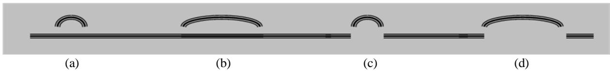
Figure 7. Schematic representation of four different characteristic Multi-Skip wall loss responses resulting from four different wall loss areas (time axis vertical and scan direction horizontal).
