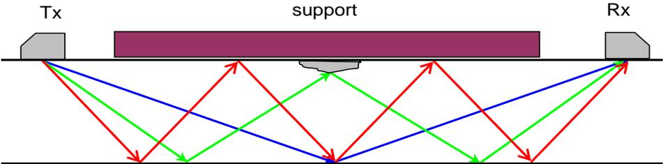
Figure 2. Basic ultrasonic Multi-Skip transmission set-up; the 1-skip (blue), 2-skips (green) and 3-skips (red) ray paths are shown.
