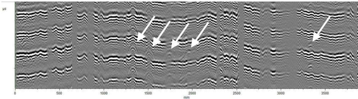
Figure 13. Full circumferential Multi-Skip scan data with local wall loss responses indicated by the arrows; longitudinal welds are located at ~700 mm and ~2550 mm.
