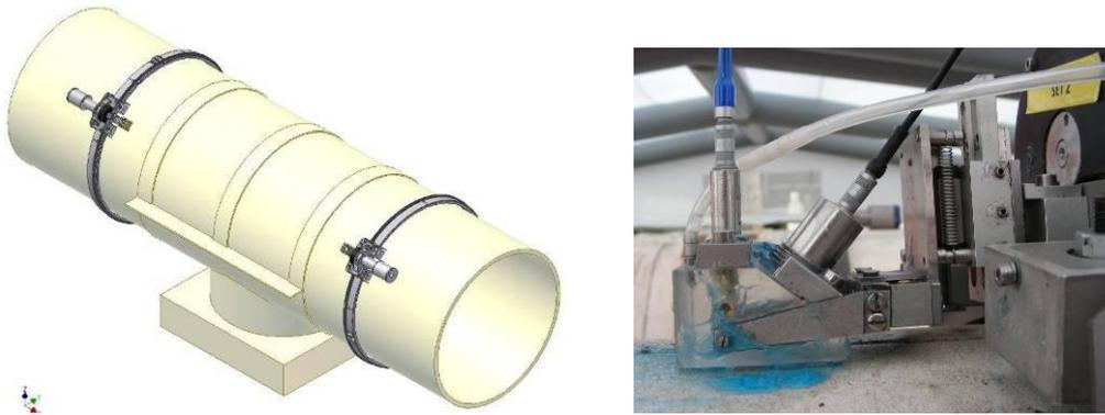
Figure 8. Multi-Skip scanner and probe assembly as developed & constructed by Sonomatic Ltd.
