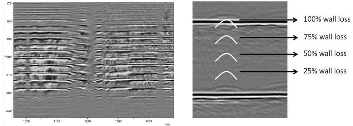
Figure 6. A ToFD representation of Multi-Skip measurements; interaction with local wall loss results in the earlier arrival of the defect signal.
