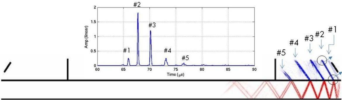
Figure 3. A snap shot of an ultrasonic wave field propagating through a plate, with the source at the left hand side; the receiver on the right hand side will record a series of (skip) signals.
