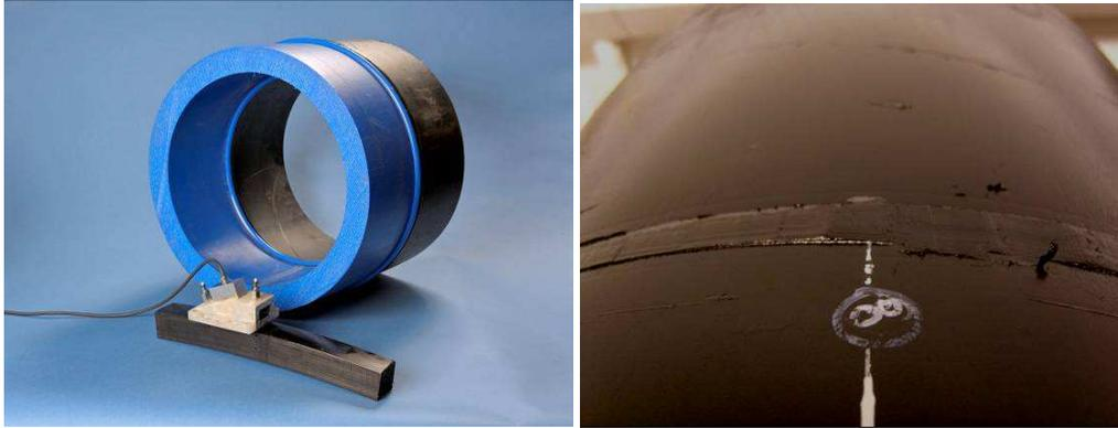
**Figure 2.** (Left) Phased array in water wedge on calibration block with test specimen and (Right) weld cap removal surface finish
